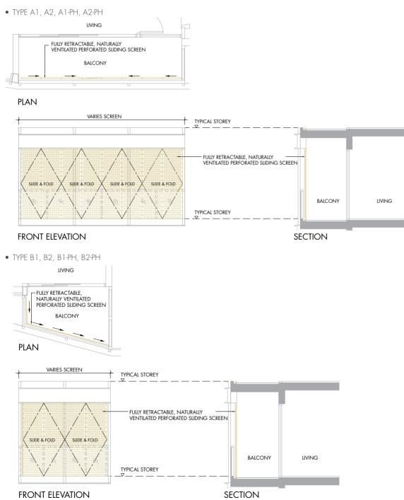
\* The screen design is provided for aesthetic uniformity of the development. Materials to be of aluminium with fluorocarbon finish. Panel design may vary for different unit types. Total free opening for perforated screen shall not be less than 50% of the panel. Drawing not to scale, and none can be regarded as representation of fact. The Purchaser is required to refer to the Management for any additional details.
